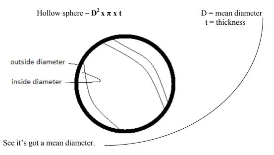
The mean diameter is half way between the outside and inside diameter, so if the outside diameter is 800mm and the material is 8mm thick there will be 8mm on the opposite side.
