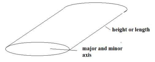
An elliptical vessel (think about the shape of the milk tanker tanks)
